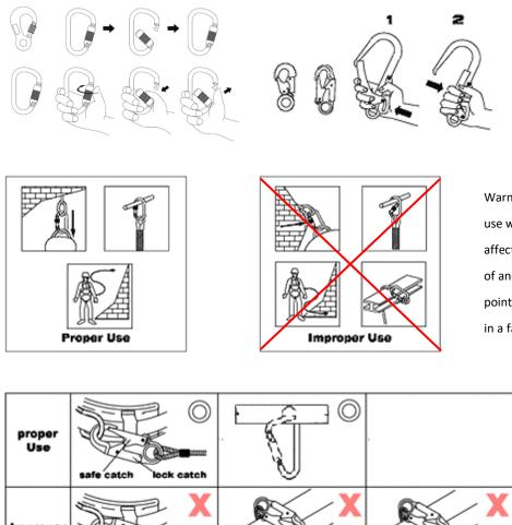
Warning: Any dangers may arise by improper use which the safe function of any one item is affected by or interferes with the safe function of another. Only connect with these proper points and a full body harness that can be used in a fall arrest system.
