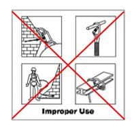
Warning: Any dangers may arise by improper use which the safe function of any one item is affected by or interferes with the safe function of another. Only connect with these proper points and a full body harness that can be used in a fall arrest system.
